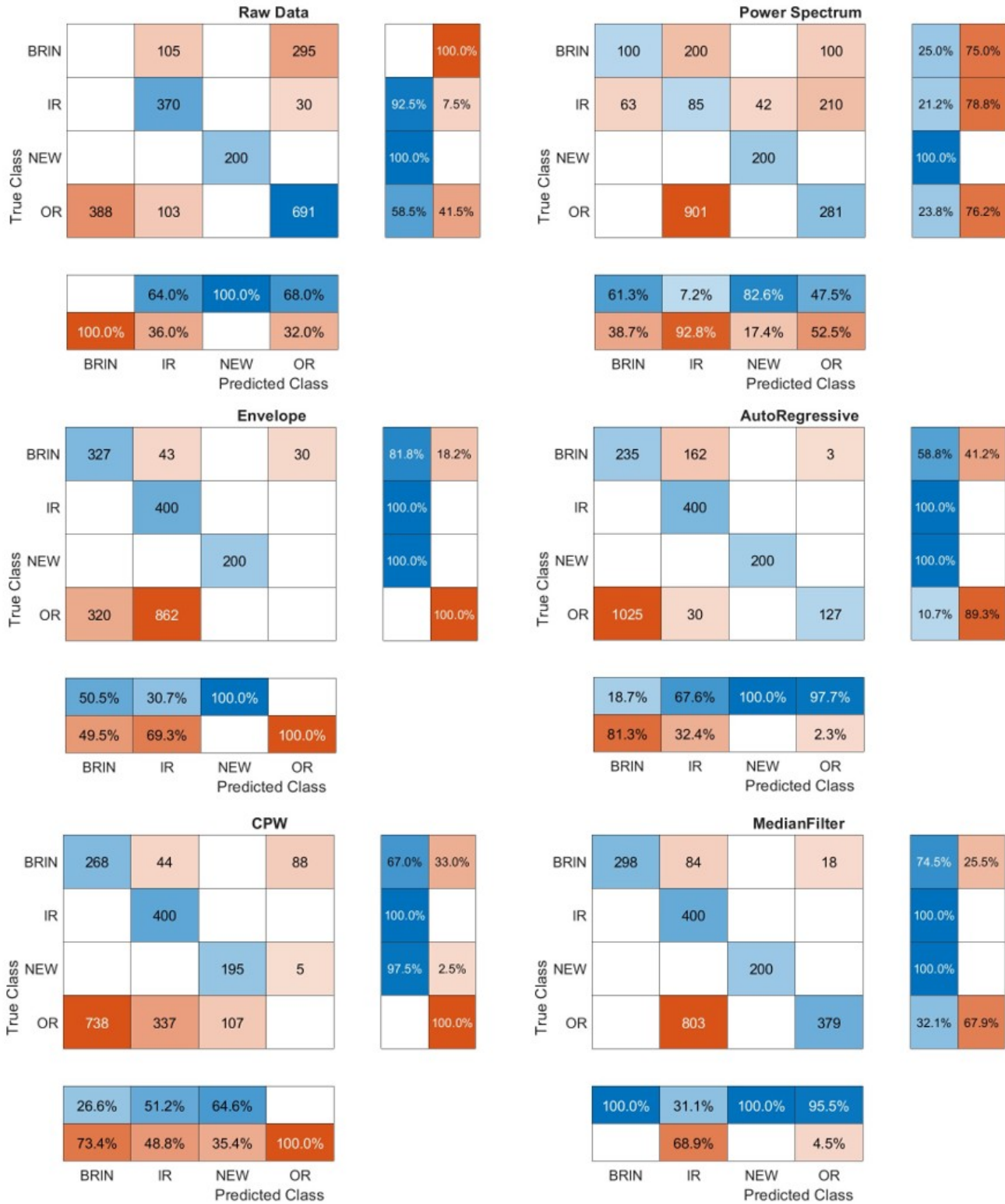
Fig. 6 Confusion matrices obtained through the validation of the trained LeNet5s for each input preprocessing strategy
