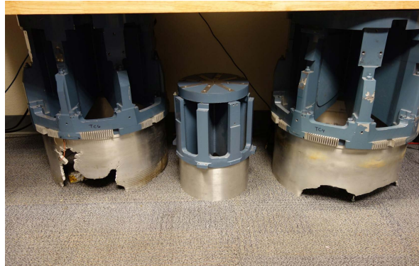
Fig. 1 Catastrophic failure due to an electrodynamic shaker being driven at a resonance in which the armature bends, leading to excessive stresses in the cylindrical part that is shown.
