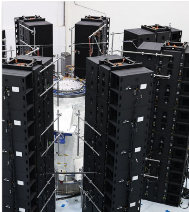
Fig. 1 Typical acoustic qualification test setup
