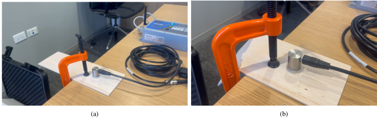
Fig. 1 The experimental setup and data acquisition system: (a) Before applying the increasing point load at the free end, and (b) After breakage/failure of the wood strip specimen
