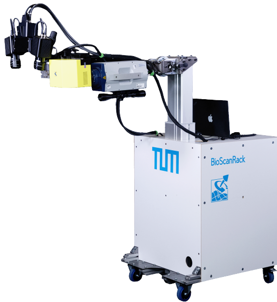
Fig. 4 BioScanRack - A mobile measurement platform with a vertical column that carries the different measurement devices.
