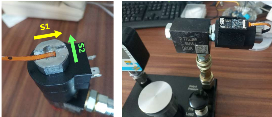
Figure 9. The sensor glued on the cap (left) and the valve at the static pressure test bench (right)
