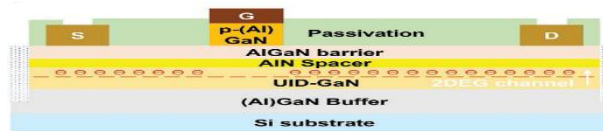
Fig-2: p-AlGa N gate enhancement-type HEMT [9].
