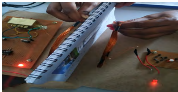
Figure 1.5 Obstruction output of the proposed work
