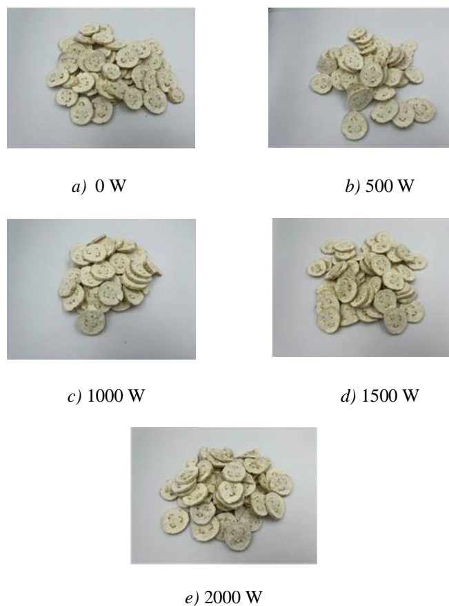
Figure 3 Dried product from different microwave power combined with hot air at 50 °C
