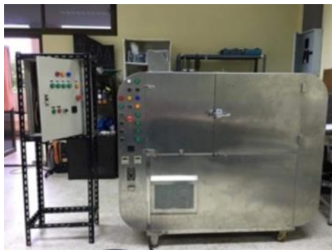
a) The pilot scale microwave assist hot air dryer
