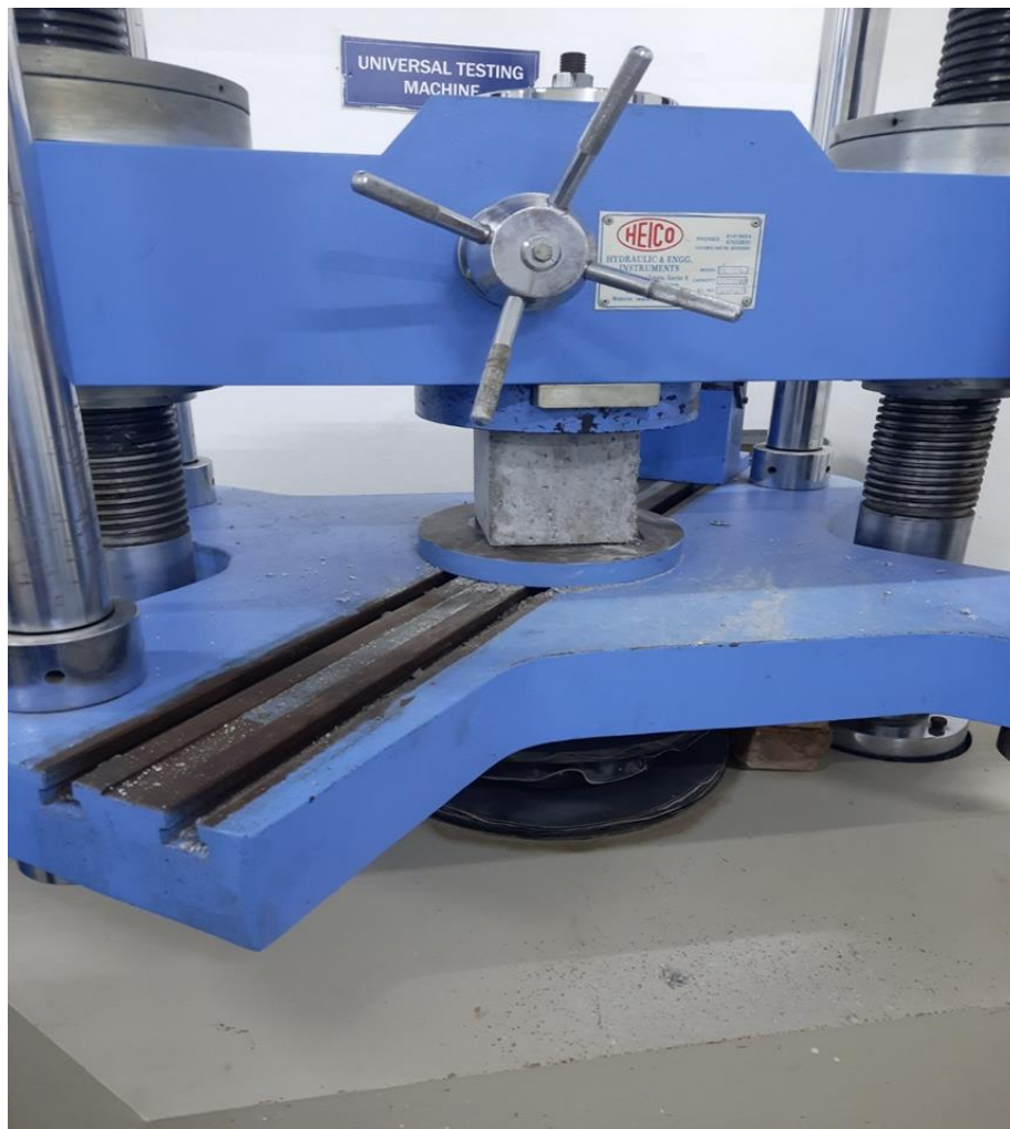
Figure 3. Experimental test for compression
