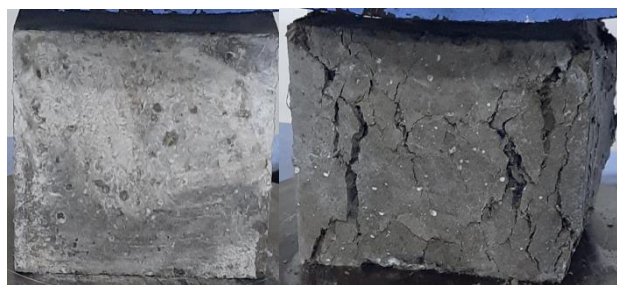
Figure 2. General crack bridging and failure mechanism
