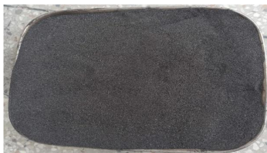
Figure 2. Raw materials image Rice husk Ash
