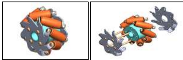
Figure 4. Proposed and exploded view of macanum Wheel
