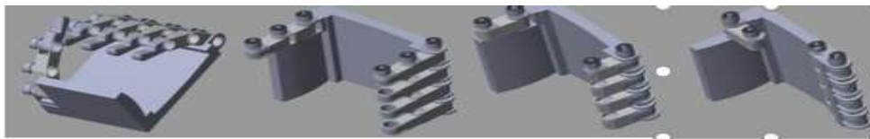
Fig. 2. Singular posture of the fingers including thumb finger and index finger
