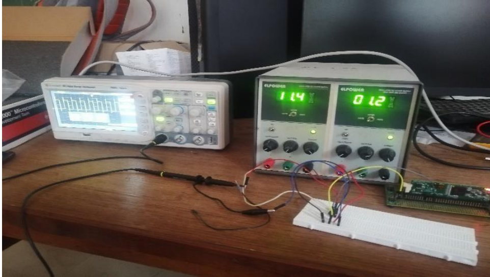
Figure 4.6. Experimental setup for MOSFET driver testing
