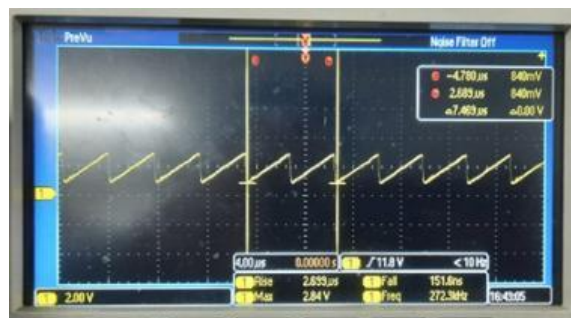
Fig.3 Saw tooth wave generated using RC network
