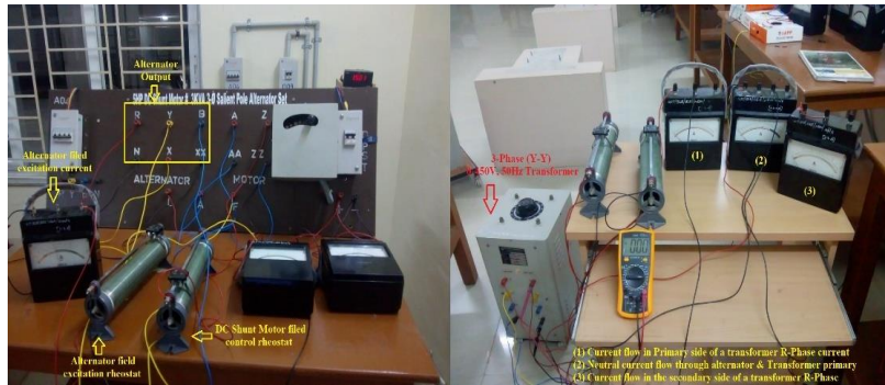
Figure 3.1 (b) Laboratory setup for Unbalanced Load on Phase-A of Transformer secondary
