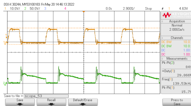
Fig 7. ■ Gate voltage and ■ Drain voltage( V_{DS} ) at 36V input
