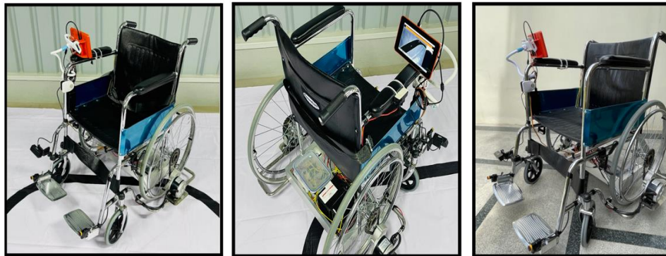
Figure 2.1. Final product: Semi-Autonomous Smart Wheelchair (left to right: wheelchair on track, top-view with active touchscreen interface, front-view)
