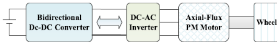
Fig.1 Use of Bi-Directional DC-DC Converter in EVs [3]
