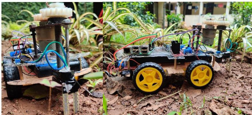
Fig. 5. Hardware model used to measure soil moisture levels in dry and wet conditions.
