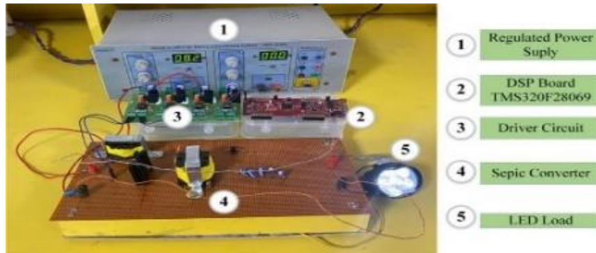
Figure 6.2. Hardware setup for dim light
