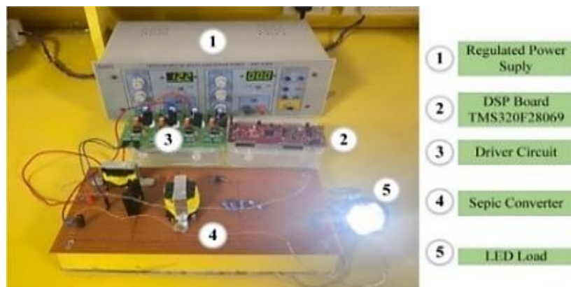
Figure 6.1. Hardware setup for bright light
