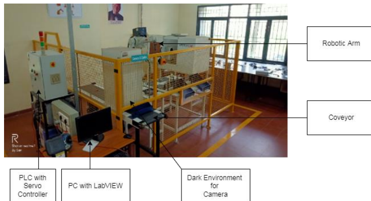
Fig 4.4 Shows the Lab setup consisting of a conveyor, a ABB Robotic Arm, PLC and Servo Controllers and a PC with LabVIEW.
