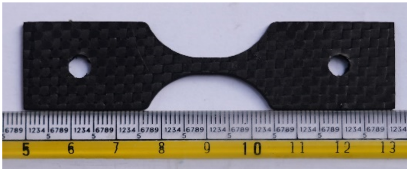
Fig. 1 Dog-bone shaped specimen for high strain rate tensile experiments
