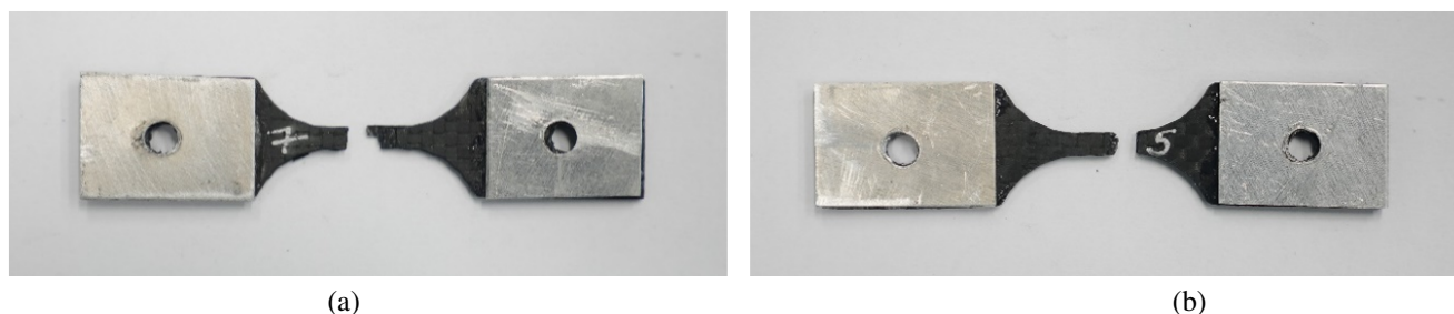
Fig. 5 Deformed specimens when subjected to (a) \dot{\epsilon} = 1466\text{ s}^{-1} at 45\text{ }^{\circ}\text{C} and (b) \dot{\epsilon} = 1630\text{ s}^{-1} at -45\text{ }^{\circ}\text{C}
