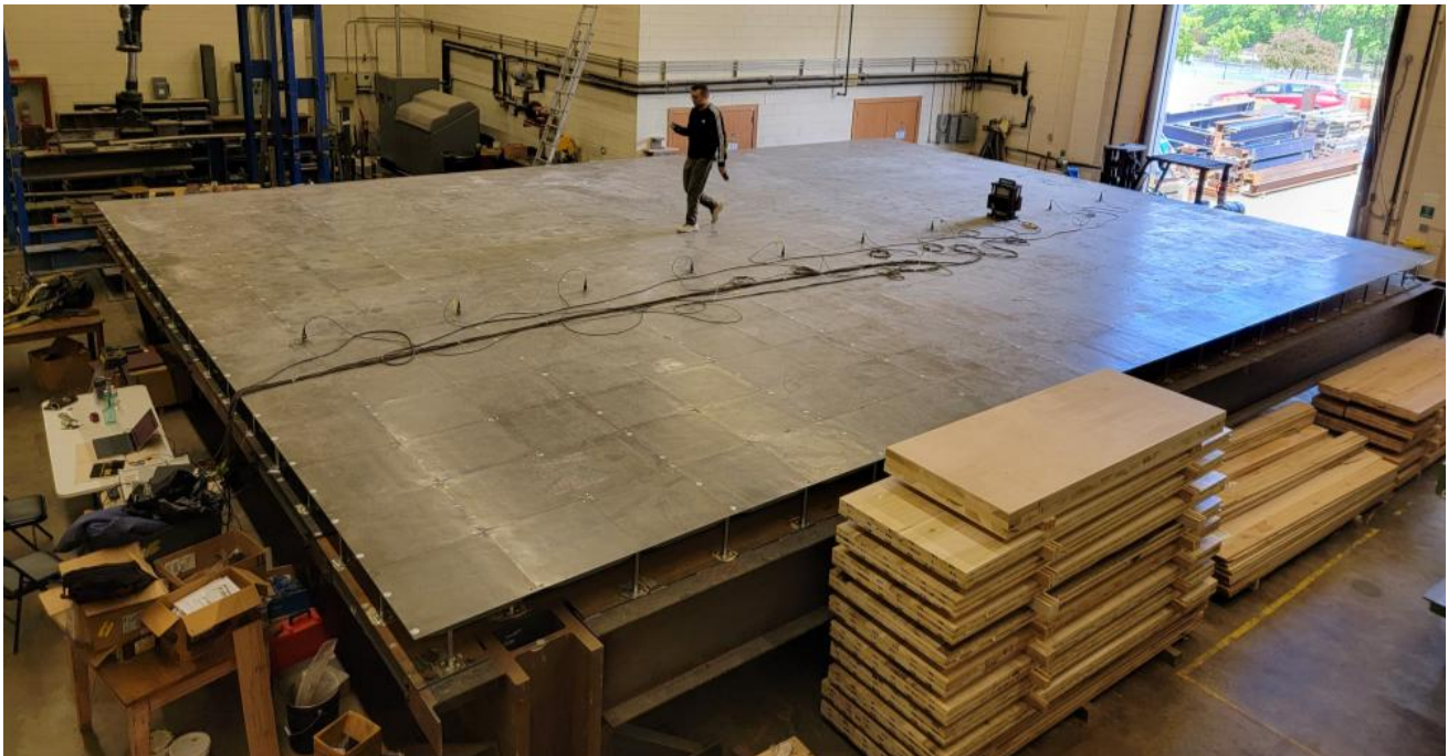
Fig. 14 Setup for the metronome-guided walking tests along the centerline of module 4, with accelerometers deployed along the centerline of module 3
