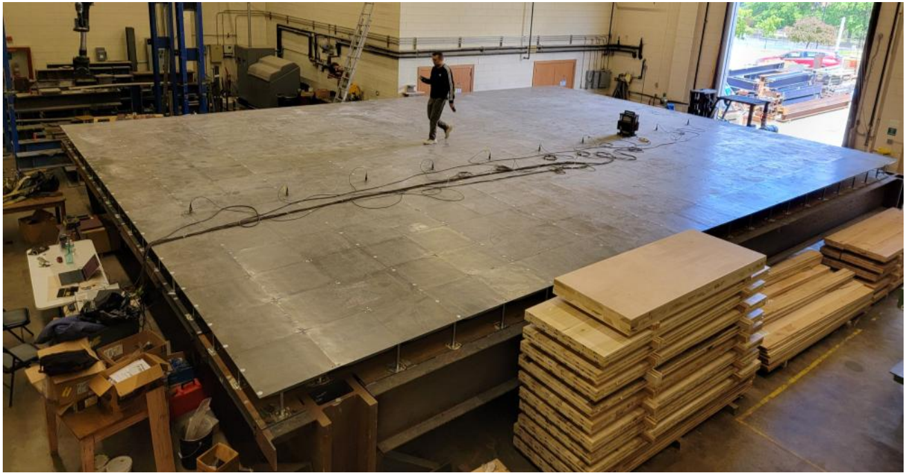
Fig. 13 Setup for the metronome-guided walking tests along the centerline of module 4, with accelerometers deployed along the centerline of module 3
