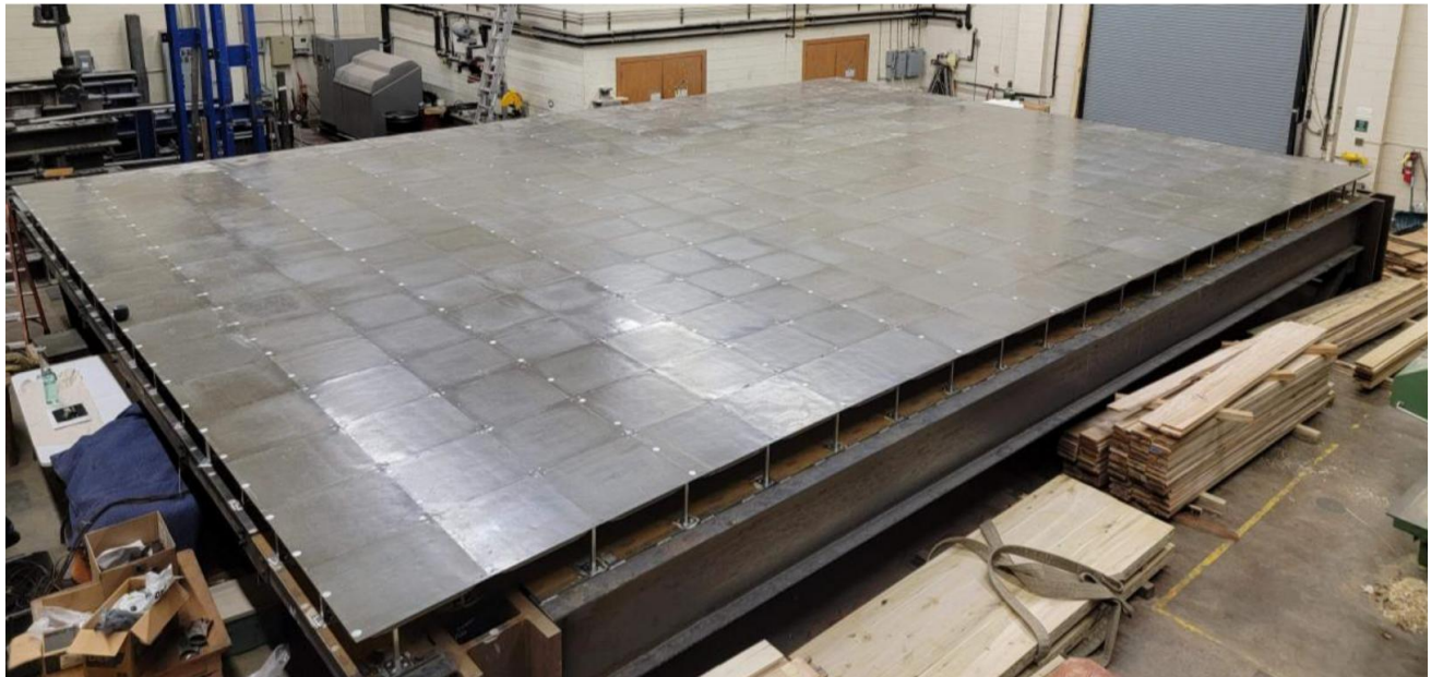
Fig. 3 The FastFloor test specimen with the raised access floor (RAF) installed
