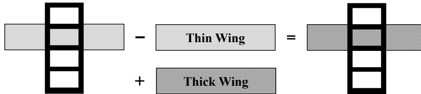
Fig. 1 A diagram of the targeted dynamic substructuring problem. The baseline structure is the thin wing bolted to the frame. We will remove the thin wing and substructure in the thick wing using the approach described in the background section.
