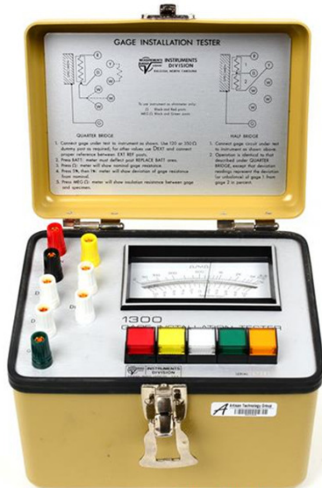
Fig. 4 Vishay Model 1300 Gage Installation Tester
