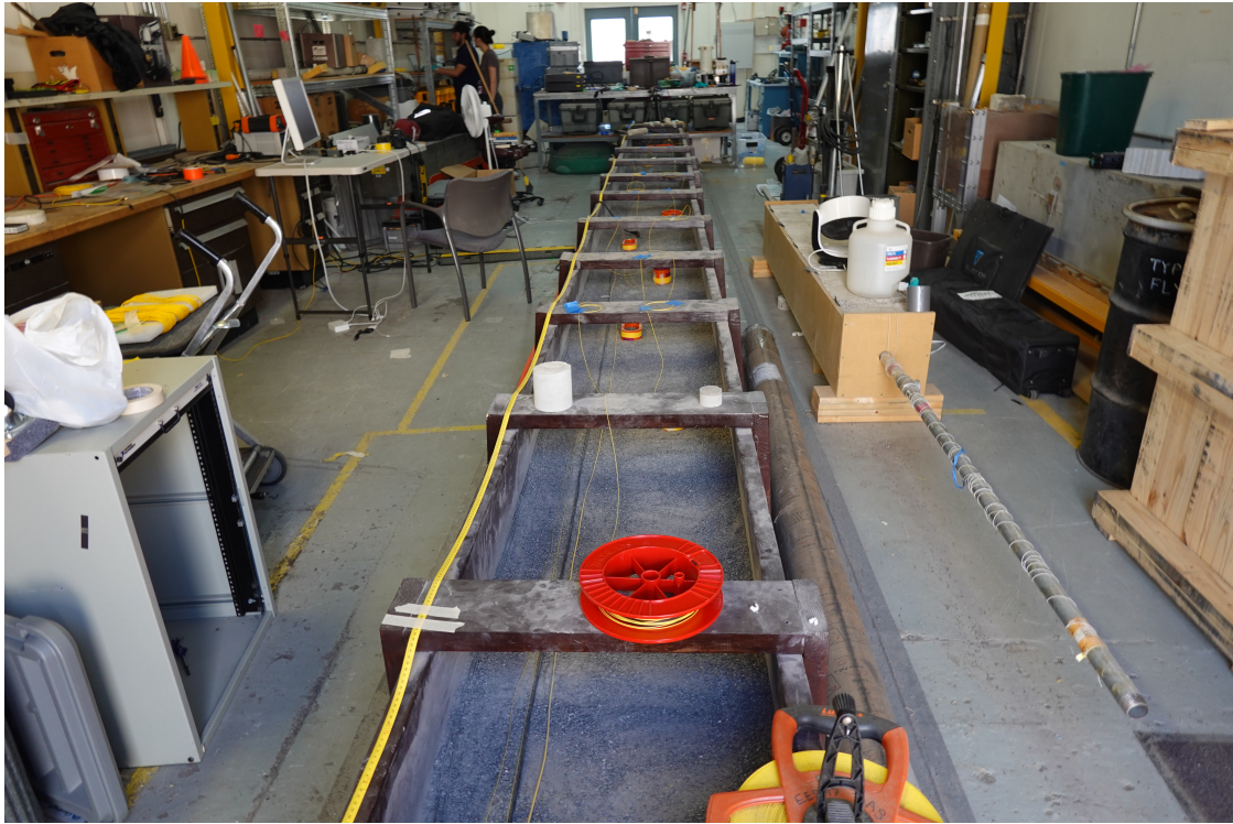
Fig. 7 The 10m long wooden box used as an indoor testing environment
