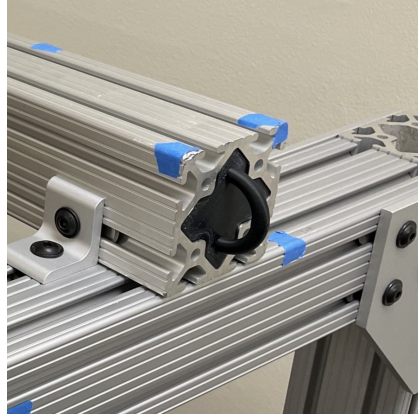
Fig. 3 Picture of beam with plastic end cap, One cap was used on each end and the cavity was filled with silica
