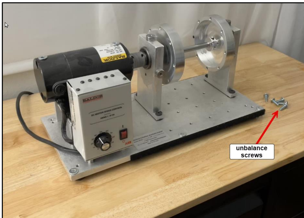
Fig. 1 Rotating Machine Showing Unbalance Screws Added to Its Rotors
