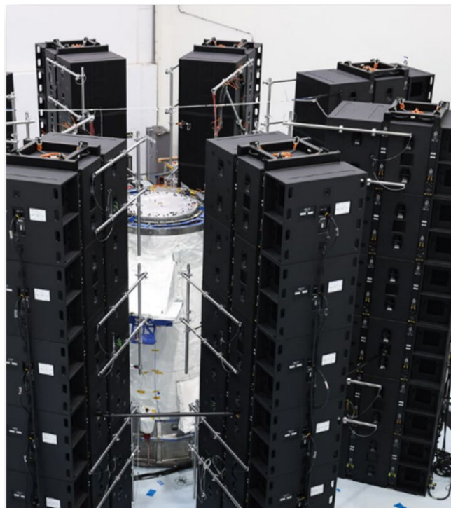
Fig. 1 Typical acoustic qualification test setup
