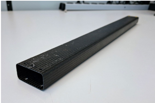
Fig. 3 Close up of the outside of the carbon fibre beam
