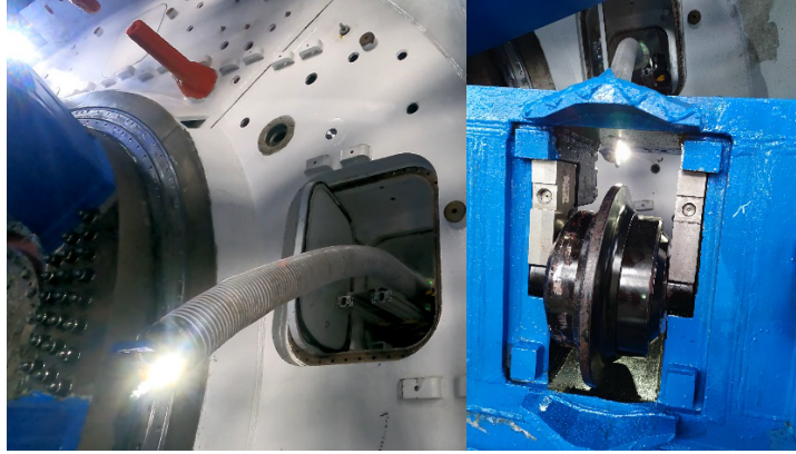
Fig. 17 The snake robot exiting the cabin for cutter inspection.
