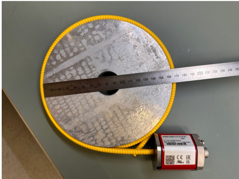
Figure 5.2: Sensor with flexible sensing element wound up in a diameter of 165 mm
