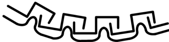
Figure 5.1: Schematic presentation of the structure of the protective tube in a bent state
