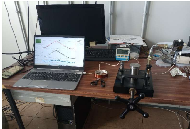
Figure 10. The static test bench (manual pressure regulation bench) and the application program for resonance frequency acquisition. Valve is mounted without coil.
