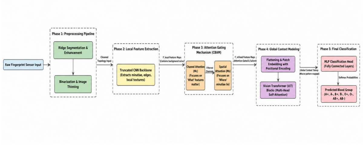
Fig. 1. Proposed workflow for fingerprint-based blood group classification.
