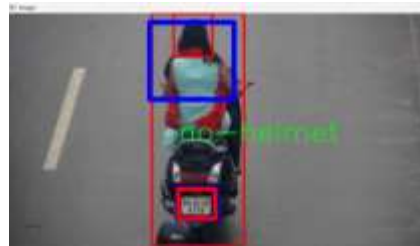
Fig. 3. The above image shows the helmet and the number plate are detected and also shows the person is not wearing the Helmet
