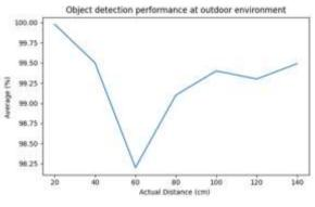
Fig. 4. Accuracy Analysis on Outdoor Object Detection
