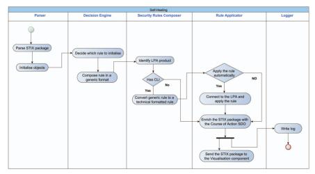
Figure 8.13 Self-healing subcomponents activity diagram.
