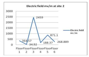
Figure 10-4 AVERAGE ELECTRIC FIELD AT A 6-STOREY BUILDING.
