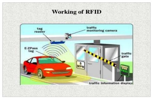
Figure 25-2 Working of RFID
