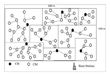
Figur 6-1 A Clustered Wireless Sensor Network
