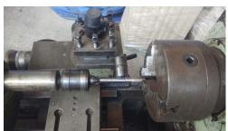
Figure 3. Burnishing tool attached to lathe tool post.
