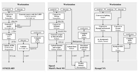
**Figure 10.2** Deployment pipelines for all platforms. From left to right: STM32L4R9, Kendryte K210 and DynapCNN. For DynapCNN, the pipeline is contained in a single Python script, while the other relay on external languages and tools.
