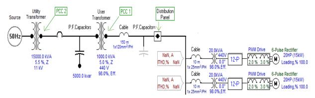
Figure 3.2.Single line configuration for simulating scenario 2
