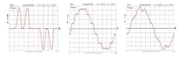
Figure 4.1.Total harmonic current waveforms of scenarios1, 2 &3 respectively
