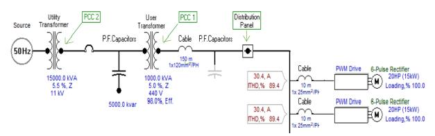
Figure 3.1.Single line configuration for simulating scenario-1
