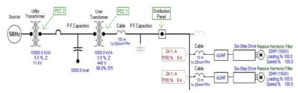
Figure 3.3.Single line configuration for simulating scenario 3
