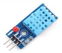
DTH 11 sensor is used in measuring the temperature, humidity and passing the information to Arduino  $% \left( {{\left[ {{{\rm{T}}_{\rm{T}}} \right]}_{\rm{T}}} \right)$
