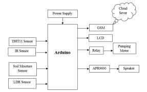
Figure 1: System Architecture
