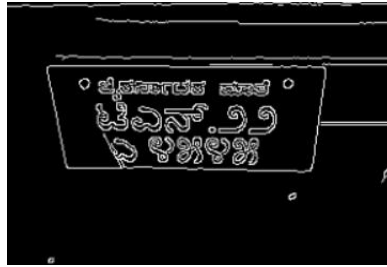
Fig. 4- Apply filter find edges for localization
