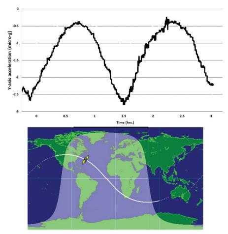
**Figure 1.1** The quasi-steady microgravity environment on the orbiter Columbia shows the effects of variations in Earth's atmospheric density. The primary contribution to the variation is the day/night difference in atmospheric density. The *plot* shows that the drag on the orbiter varies over a ninety-minute orbit (Courtesy NASA, 1997 [2]).
