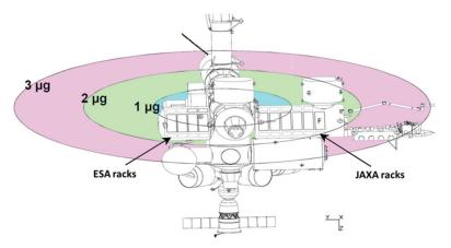
**Figure 1.3** Self-gravitation in the International Space Station (*ISS*). Depending on the location with the ISS mass perceives a gravitational pull ranging from 0 to  $3 \times 10^{-6}$  g from the total mass of the ISS itself [4] (Image courtesy NASA).
