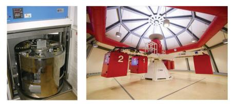
**Figure 11.1** Two examples of research centrifuges. *Left* The medium-diameter centrifuge for artificial gravity research (MidiCAR) is a 40-cm-radius system for (mainly) cell biology research [16]. *Right* The large-diameter centrifuge (LDC) [6] is an 8-meter-diameter system used for life and physical sciences and technological studies. Both centrifuges are located at the TEC-MMG Lab at ESA-ESTEC, Noordwijk, The Netherlands.
