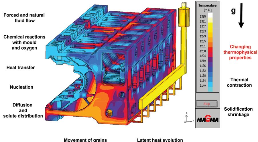
**Figure 21.1** A wide range of fundamental events during casting of complex components, here a car engine with varying local temperatures.
