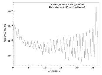
**Figure 3.3** Measured spectra of fragments produced by a beam of 1 GeV/n Fe-ions on a target of 26 mm Al. Fragments at 0 degree are measured by a Si-telescope. Each peak correspond to a fragment of a different atomic number Z. Measurement performed at the Brookhaven National Laboratory (NY, USA), courtesy of Jack Miller and Cary Zeitlin, Lawrence Berkeley National Laboratory, CA, USA.
