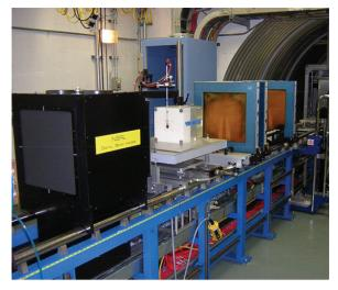
**Figure 3.2** Irradiation facility at NSRL in Upton, NY, USA. The facility is dedicated to the NASA Space Radiation Health Program, the largest research program in the field of simulation of cosmic radiation effects. The photograph showing three large monitor chambers, a plastic target, the egg chamber used for dose measurements, and the digital beam analyzer to check beam position and uniformity. Image from the NSRL Web site [7].
