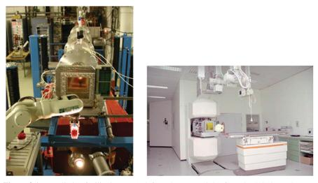
**Figure 3.1** Irradiation facility in cave A (left) and cave M (right) from the SIS18 synchrotron of the GSI Helmholtz Center in Darmstadt, Germany. Cave A is equipped with a robotic arm for remote control of the samples. Cave M is equipped with a couch used in 1997–2008 for treatment of cancer patients with C-ions and is currently dedicated to experiments in animals or other 3D targets. Image from the GSI Web site [6].
