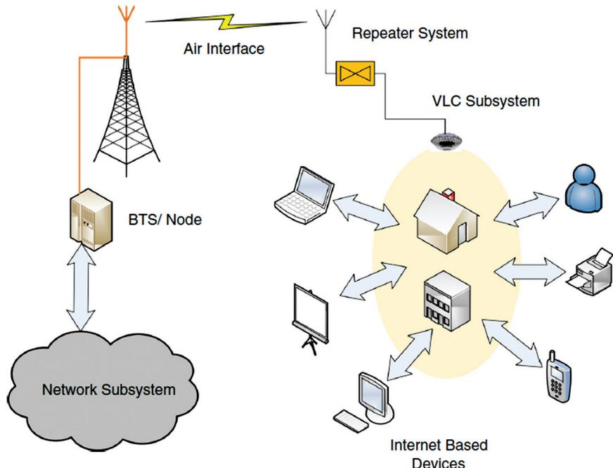
**Figure 1.3** VLC system architecture.
