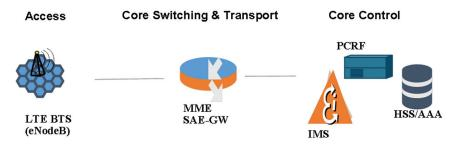
Figure 10.6 LTE/SAE system architecture (Picture NSN).
