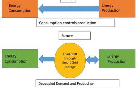
Figure 10.12 Consumption controls production and decoupled demand and production.
