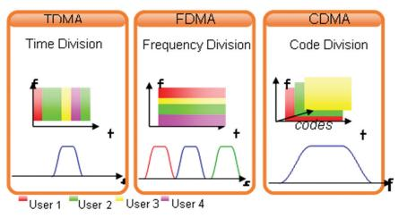
Figure 10.3 Major multiple access methods used in 2nd and 3rd mobile radio standards (Picture NSN).
