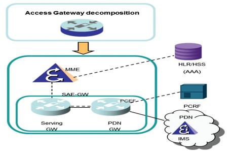
Figure 10.8 Core network principles (Picture NSN).
