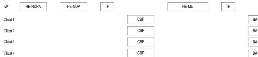
Figure 12.9 Downlink and uplink MU for 11ax.
