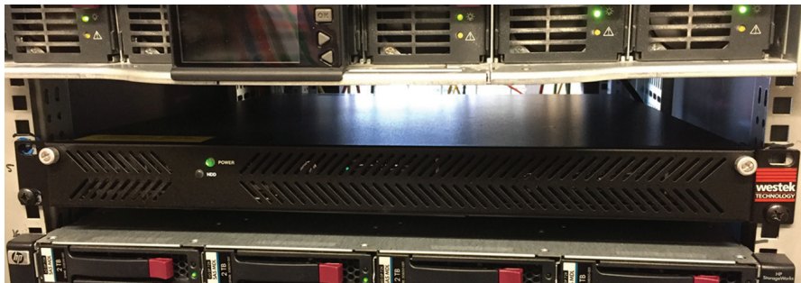
Figure 9.5 IP-based digital exchange for ship-to-shore radio anno 2016.
