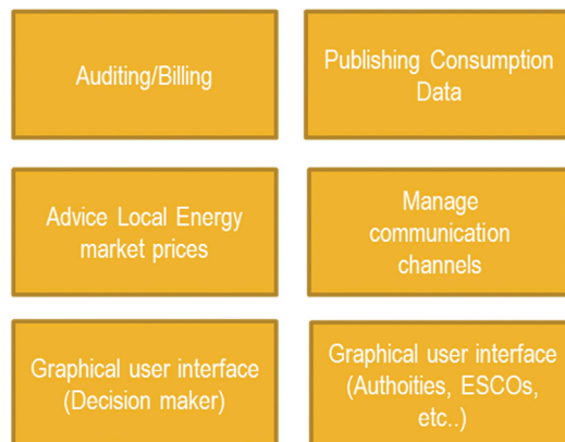
Figure 2.14 CDSS HMI sub-component.
