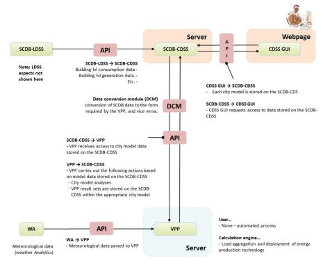
Figure 6.1 iURBAN ICT architecture—CDSS/VPP relationship diagram.
