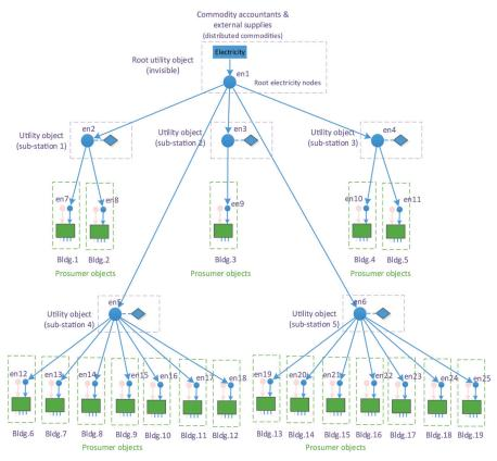
Figure 6.10 Simple VPP electricity network model—Rijeka, Croatia.
