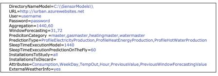
Figure 7.5 config.properties file example.
