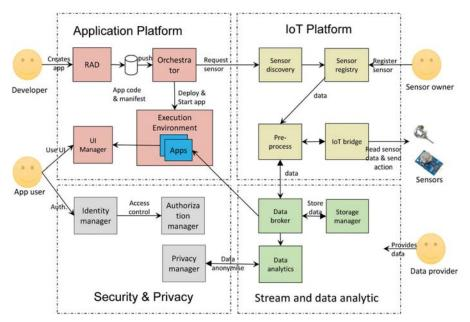
Figure 24.3 Components of the WAZIUP platform.
